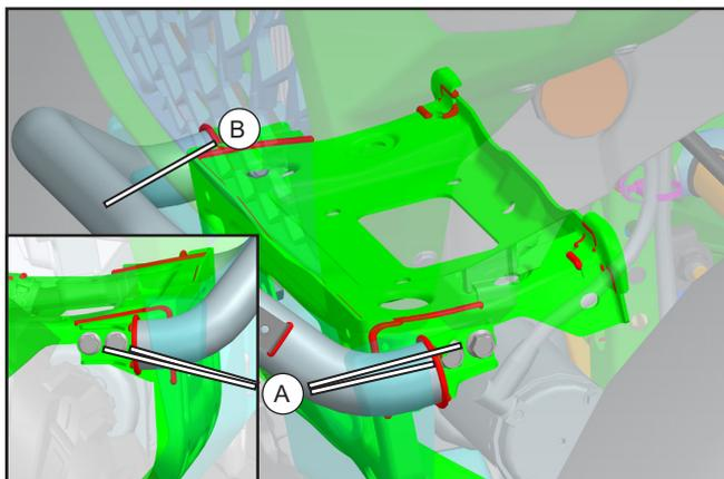
// Unscrew four M8x16 bolts (A), then take out the original front bumper (B).
