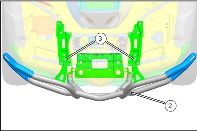
// Place the Front Bumper Assembly (2) into position, then install and finger-tighten two M8x16 bolts (3) to secure the bumper on the frame sheet metal. *Do not fully tighten at this time.*
