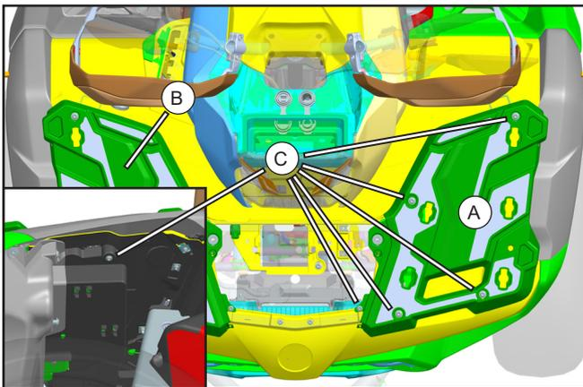
// Remove the six screws (C) from each front rack panel (A, B), then remove the panels.
