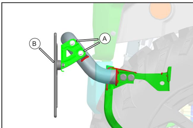
// **(B) - if equipped:** Unscrew two M6x12 bolts (A), then take out the front license frame.
