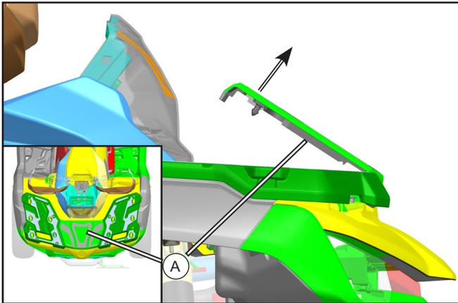
// Pull up the front service cover (A) in the arrow direction shown and remove it.
