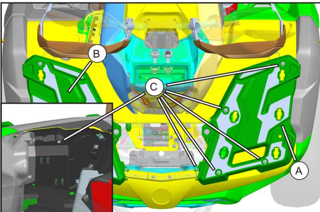
// Reinstall LH and RH front rack panels (A,B), then secure them with the removed screws (C).
